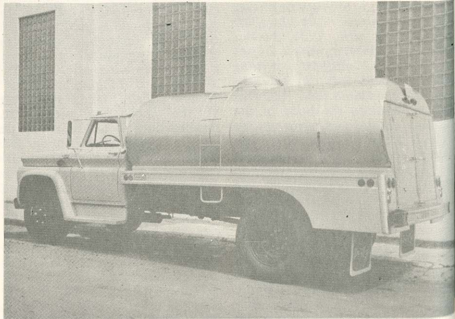
A REFRIGERATED MILK TRUCK USED TO DELIVER MILK FROM FARM TO THIEL BROTHERS FACTORY AT SHERWOOD.
